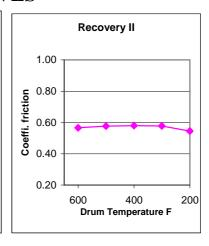
\*Note 1. – Friction values shown are for guide purposes only since values deviate with changes in temperature, pressure and speed. Practical design should include a 25 to 50 percent safety factor.
