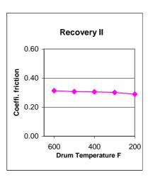
\*Note 1. – Friction values shown are for guide purposes only since values deviate with changes in temperature, pressure and speed. Practical design should include a 25 to 50 percent safety factor.
