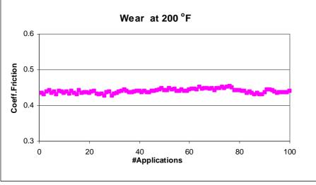
Wear Test Parameters: Speed 411 RPM, Load 150 LB, Temperature 200°F, Cast Iron drum Diameter 278 mm \*Note 1. – Friction values shown are for guide purposes only since values deviate with changes in temperature, pressure and speed. Practical design should include a 25 to 50 percent safety factor.
