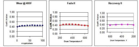
\*Note 1. – Friction values shown are for guide purposes only since values deviate with changes in temperature, pressure and speed. Practical design should include a 25 to 50 percent safety factor. \*\*Note 2. – Rubbing speed, drum temperature, and pressure are directly related. Changing any one value will change the others.
